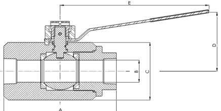
Pressure Class 900# Max Working pressure: 2000 psi with suitable soft trim.
